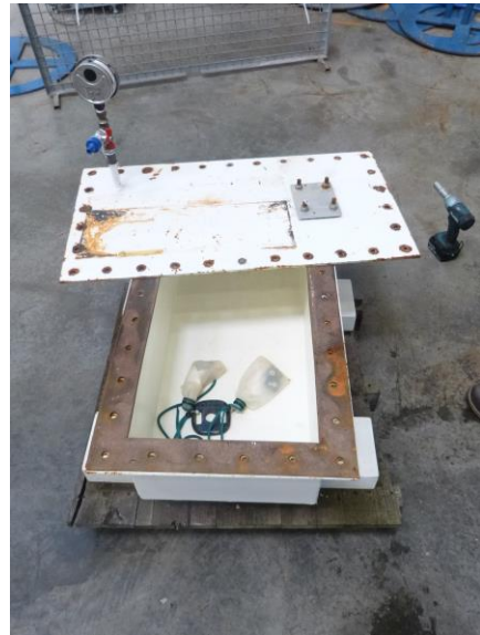
Sealed vessel for IPX8
